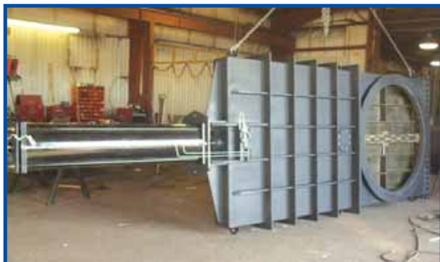
66" Zero Leakage Gate Valve (2)
