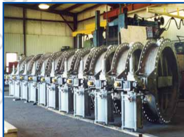
48" Pneumatically Operated Tadpole Butterfly
