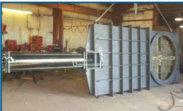
66" Zero Leakage Gate Valve (2)
